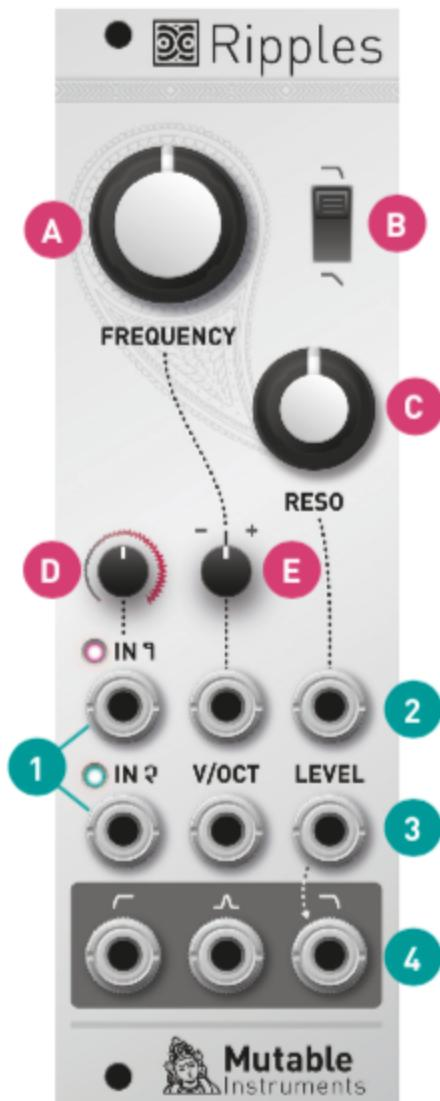
**A. Cutoff frequency.** From 20Hz to 20kHz.
